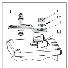
Fig. 5-1: Changing the pin position or exchanging the lever
