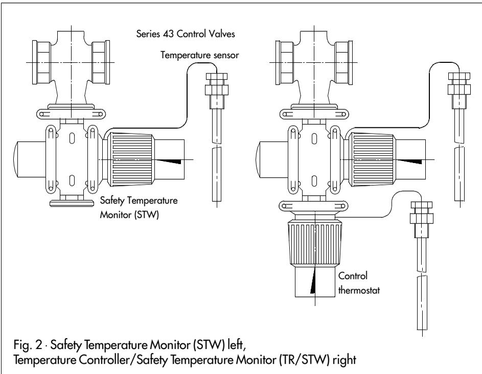
Fig. 2 · Safety Temperature Monitor (STW) left,
