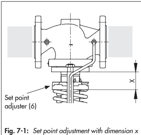
Fig. 7-1: Set point adjustment with dimension  $x$
