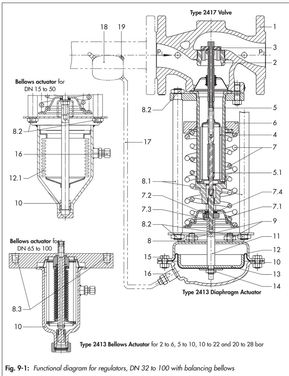
Fig. 9-1: Functional diagram for regulators, DN 32 to 100 with balancing bellows
