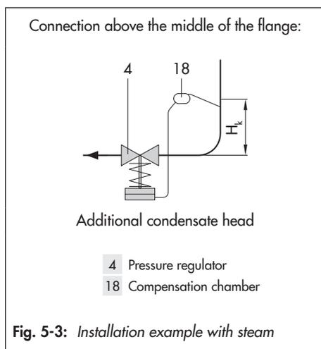
**Fig. 5-3: Installation example with steam**
