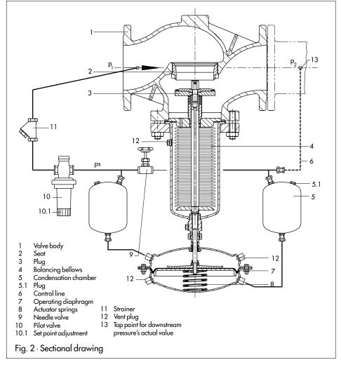
ferential pressure  $(p_s - p_2)$  to rise again and the valve plug also moves in the opening direction until the set point is reached.
