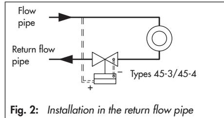
The differential pressure creates a positioning force at the operating diaphragm which moves the valve plug depending on the force of the set point spring(s) (8/10).
