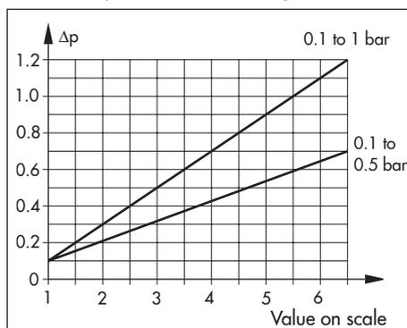
Fig. 4: Set point adjusted according to the value on the scale
