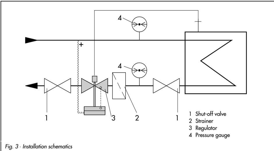
Fig. 3 · Installation schematics
