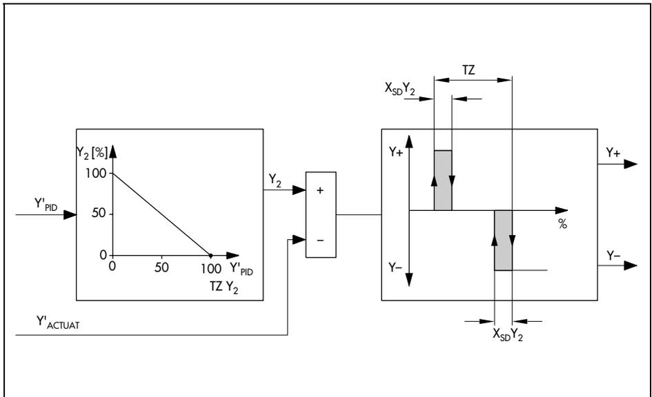
Fig. 45 · Three-step output with external position feedback
