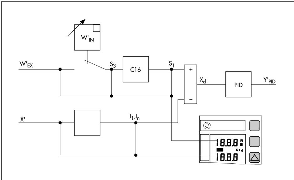
Fig. 75 · Digital displays in follow-up control mode
