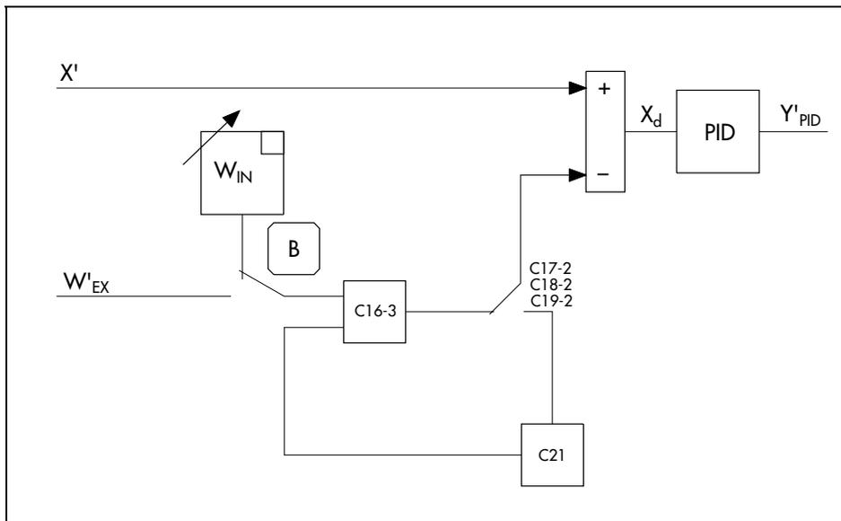
Fig. 55 · Reference variable ramp without starting condition
