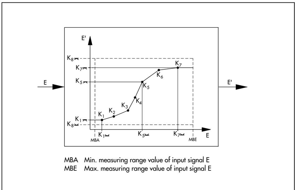
Fig. 6 · Graphical representation of function generation
