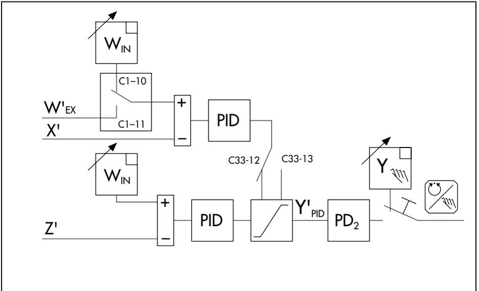
Fig. 28 · Limiting control with limited  $Y_{PID}$
