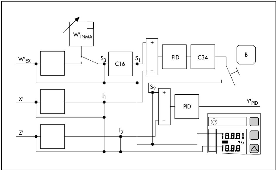
Fig. 77 · Digital displays in cascade control mode
