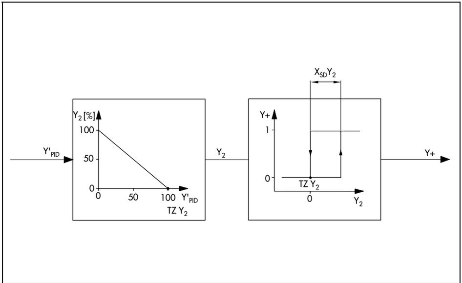
Fig. 42 · On-off output selected via C5-4
