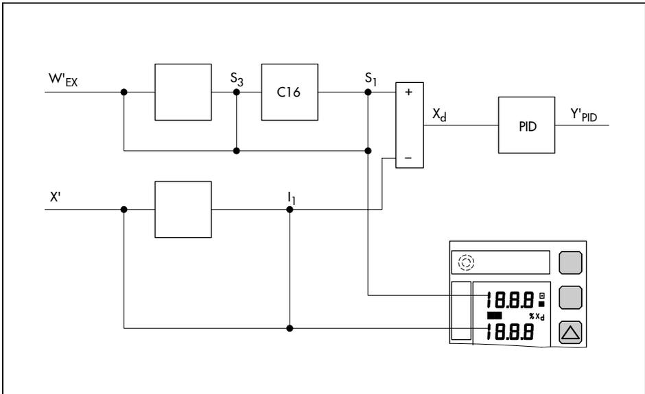
Fig. 78 · Digital displays in synchro control mode
