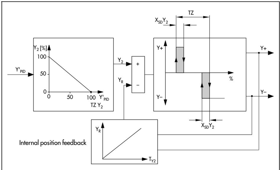
Fig. 46 · Three-step output with internal position feedback
