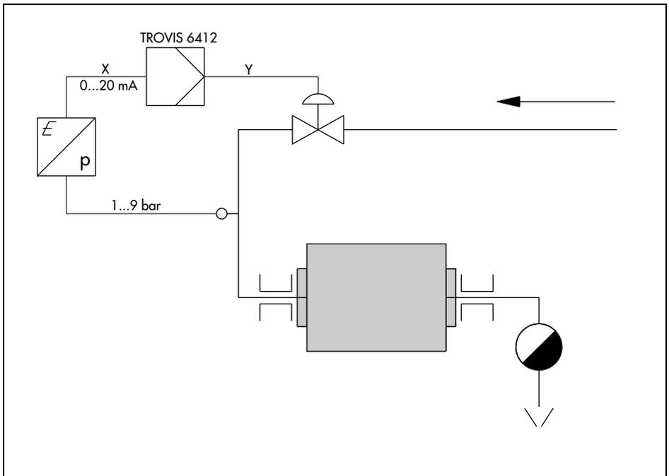
Fig. 8 · Temperature control of a calender bowl
