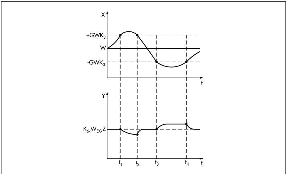
Fig. 71 ·  $Y_0/PI(D)$  change of control action
