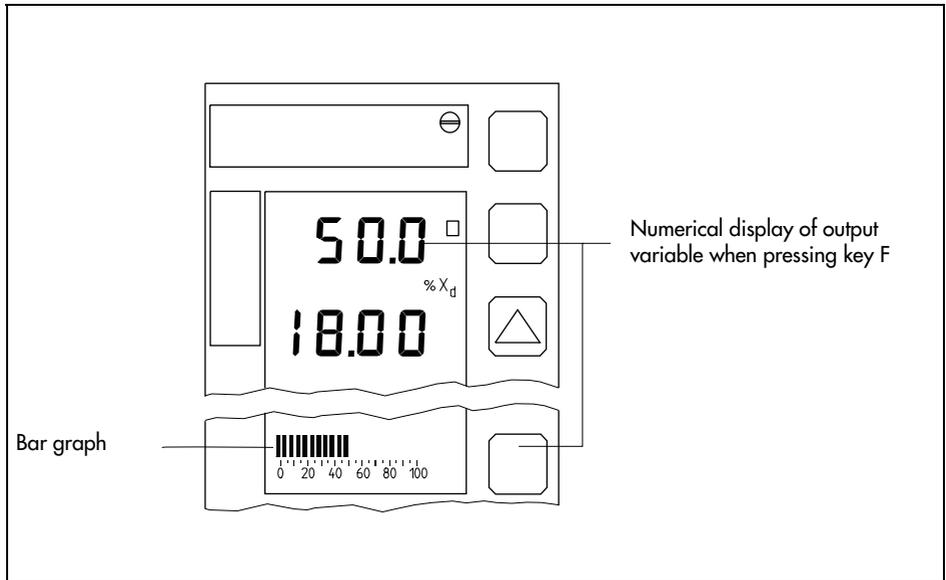
Fig. 79 · Assignment of output variable display
