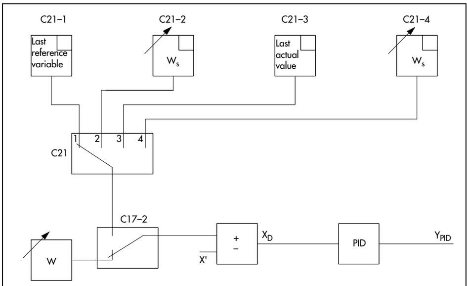
Fig. 11 · Reference variable changeover via binary input
