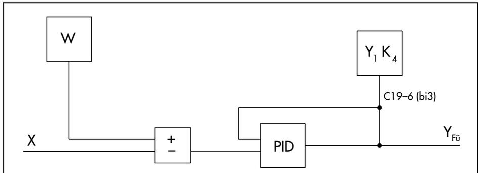
Fig. 16 · Activation of safety output value  $Y_1K_4$
