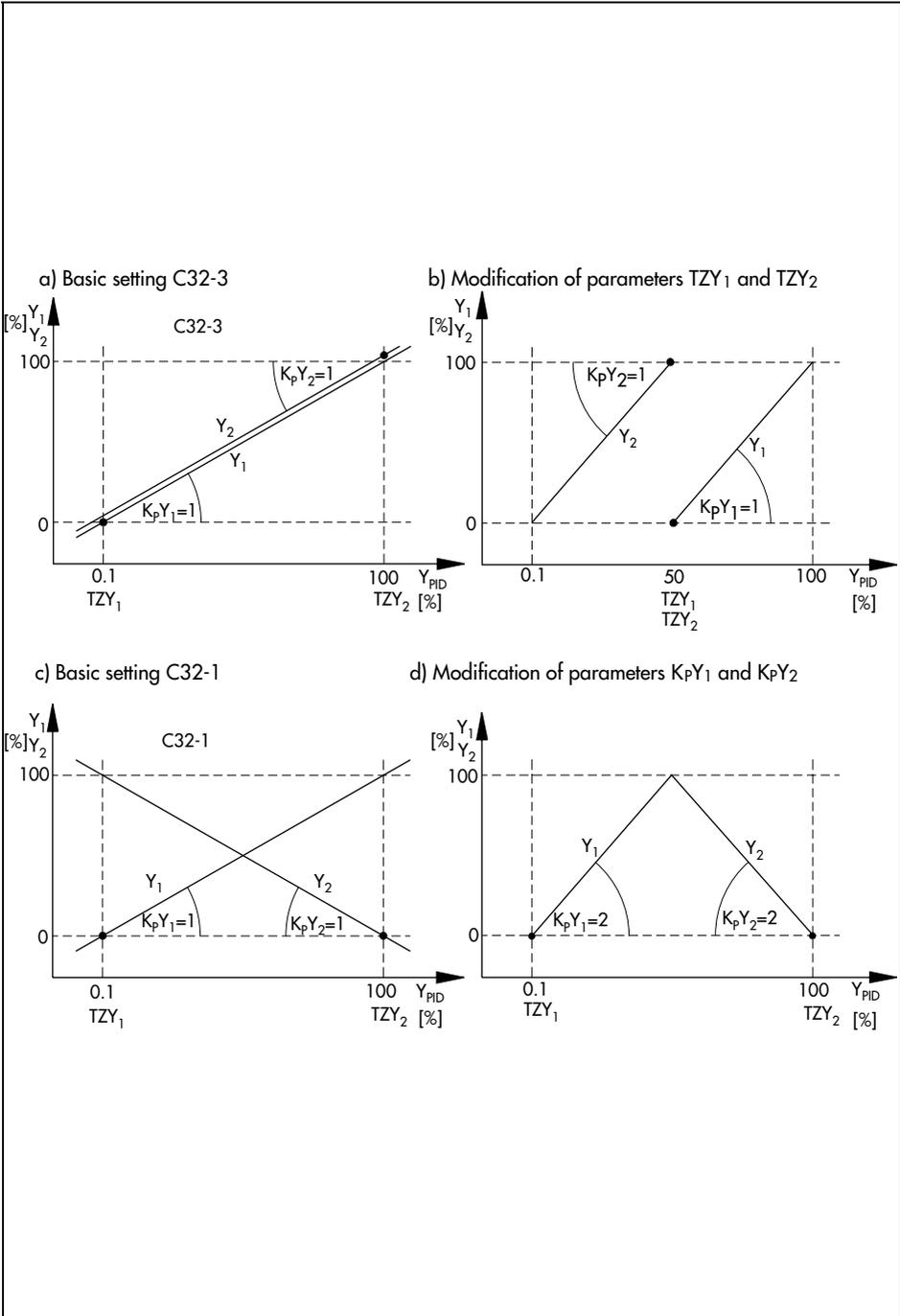
Fig. 50 · Examples for the setting of characteristics
