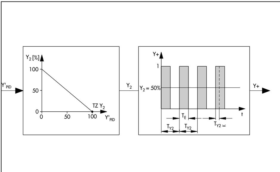
Fig. 44 · On-off output with PP converter
