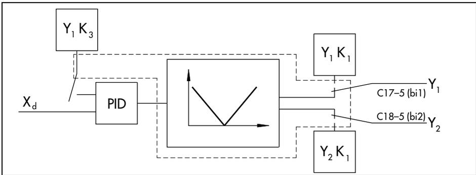
Fig. 14 · Activation of safety output value  $Y_1K_3$
