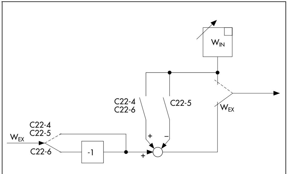
Fig. 59 · Assignment of internal reference variable via C22-4/-5/-6
