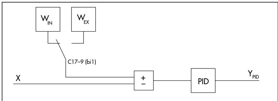
Fig. 19 · Reference variable changeover via binary input 1
