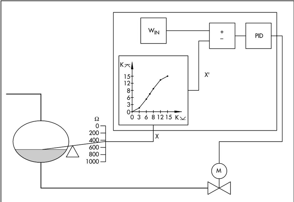
Fig. 9 · Function generation of the liquid level
