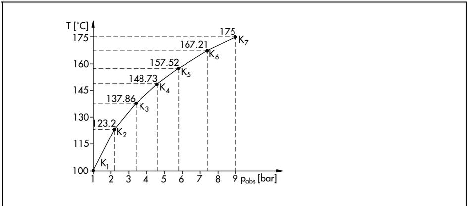
Fig. 7 · Pressure-temperature curve of example 1 for function generation
