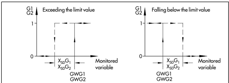
Fig. 52 · Functioning of limit relays G1 and G2
