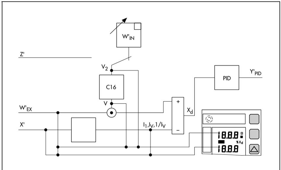
Fig. 76 · Digital displays in ratio control mode
