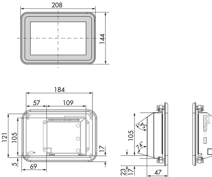
Fig. 4: Dimensions of TROVIS 6616 Web Terminal
