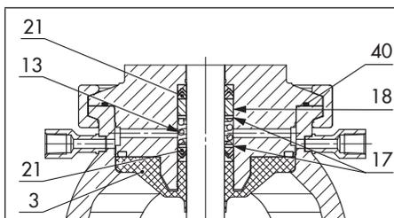
**Fig. 9-9:** DN 100 to 125 · Bar stock body · Version with steam barrier and PTFE seal: plug stem seal (without centering ring)
