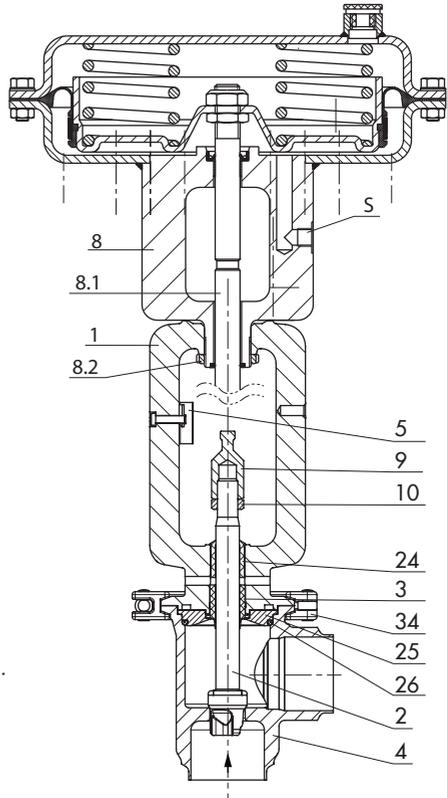
**Fig. 3-2:** (right) Sectional drawing of Type 3347-7 Control Valve (with Type 3277 Actuator) - Cast body with PEEK seal
