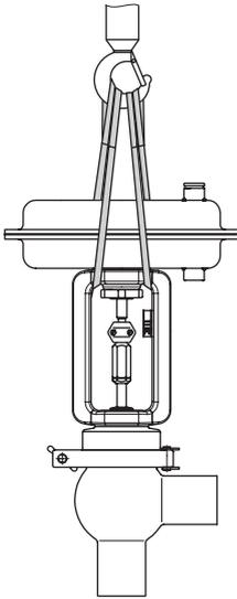
**Fig. 4-1:** Type 3347 with Type 3271 without lifting eyelet
