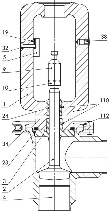
**Fig. 9-13:** DN 25 to 100 · Cast body · Version without steam barrier, with plug stem seal (without centering ring)
