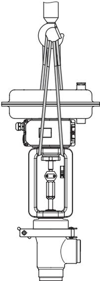
**Fig. 4-3:** Type 3347 with Type 3277 without lifting eyelet
