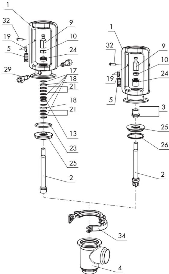
Bar stock body with anti-crystallizing seal
