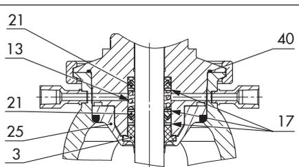
**Fig. 9-8:** DN 65 to 80 · Bar stock body · Version with steam barrier and PEEK seal: plug stem seal and metal centering ring
