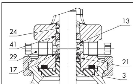
**Fig. 9-11:** DN 15 to 50 · Bar stock body · Version with PTFE packing and stopper (without steam barrier), with PTFE plug stem seal (without centering ring)
