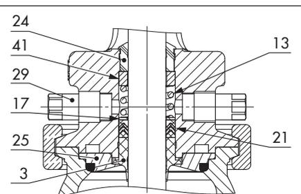
**Fig. 9-12:** DN 15 to 50 · Bar stock body · Version with PTFE packing and stopper (without steam barrier), with PEEK plug stem seal and metal centering ring
