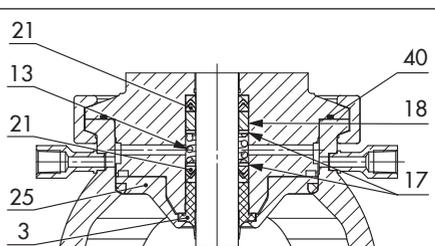
**Fig. 9-10:** DN 100 to 125 · Bar stock body · Version with steam barrier and PEEK seal: plug stem seal and metal centering ring
