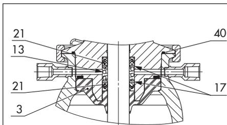
**Fig. 9-7:** DN 65 to 80 · Bar stock body · Version with steam barrier and PTFE seal: plug stem seal (without centering ring)
