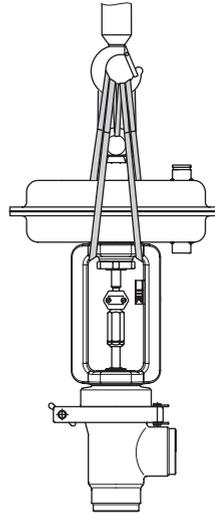
**Fig. 4-2:** Type 3347 with Type 3271 with lifting eyelet
