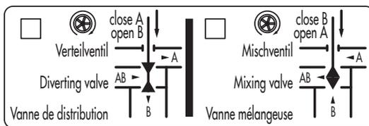
Fig. 4: Label on handwheel when mounted on SAMSON three-way valves
