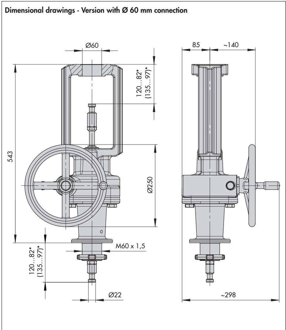
\* For "Actuator stem retracts" direction of action: swap top and bottom stem connector nuts
