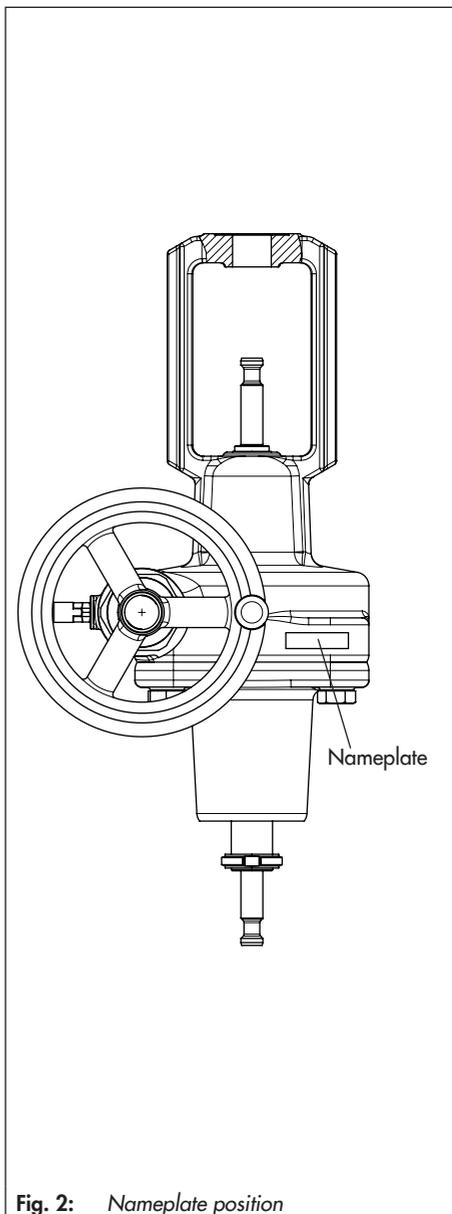
**Fig. 2:** Nameplate position
