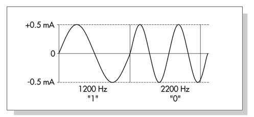
Fig. 33: FSK-coded data transmission based on Bell 202 (half-duplex)
