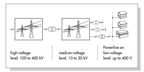
Fig. 34: Powerline uses low-voltage power supply network
