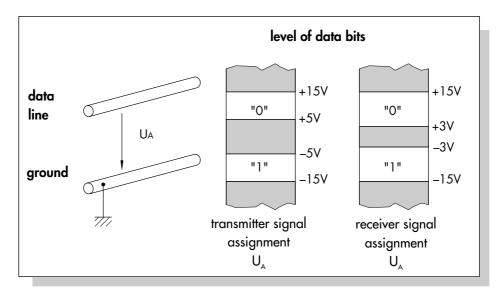
Fig. 26: RS 232 transmitter and receiver level
