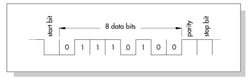
Fig. 19: Asynchronous transmission using the UART character (universal asynchronous receiver transmitter)
