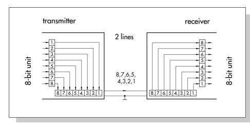
simple two-wire line for bit-serial data transmission
