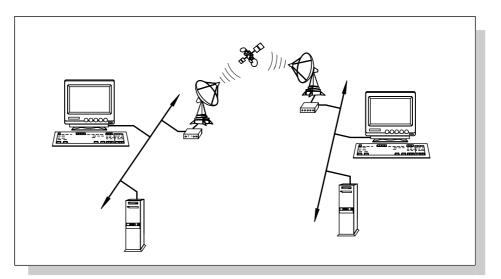
Fig. 13: Connection of networks via satellite telecommunication link
