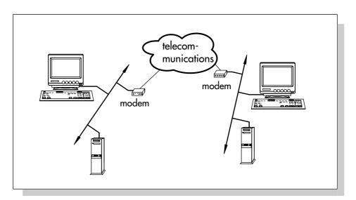
Fig. 35: Modems as coupler between telephone and digital network
