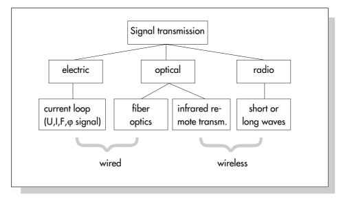
Fig. 6: Media for serial data transmission
