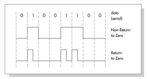
Fig. 15: NRZ and RZ coding with positive logic
