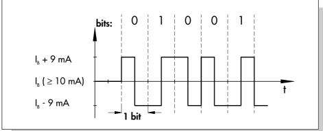
Fig. 32: IEC 61158-2 with Manchester coding using  $\pm 9$  mA
