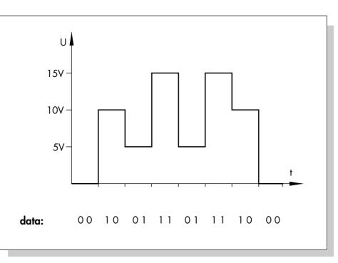
Fig. 5: More complex encoding reduces transmission frequency
