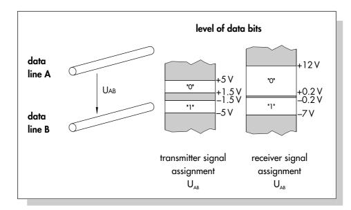
Fig. 29: Signal level of balanced RS 422 interface
