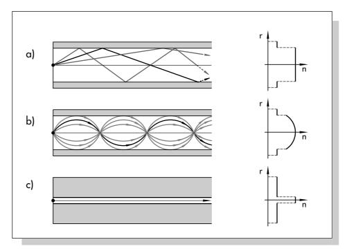
Fig. 12: Profiles and refractive indices of optical fibers
