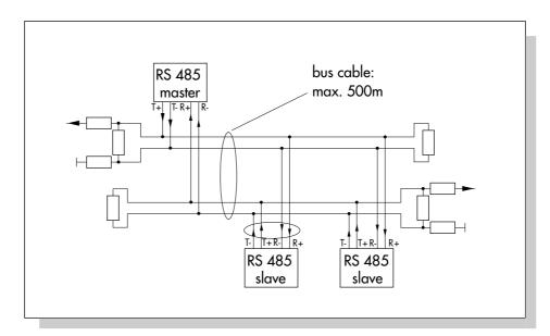
Fig. 31: 4-wire connection with RS 485 interface (master/slave communication)
