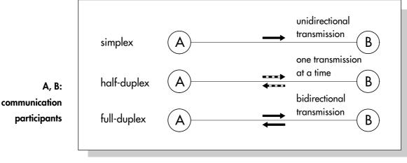
Fig. 2: Different communication techniques
