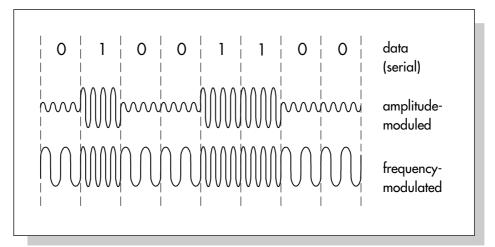
Fig. 17: Encoding by means of amplitude and frequency modulation
