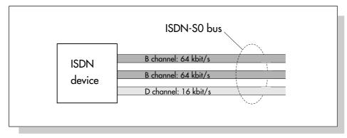
Fig. 36: Data channels of an ISDN connection
