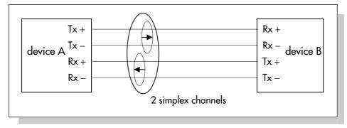
Fig. 27: 4-wire full-duplex connection with RS 422 wiring
