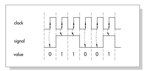
Fig. 18: Synchronous signal sampling with positive edges
