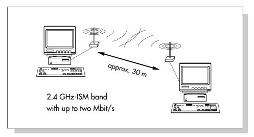
Fig. 14: Simple WLAN for use in the domestic field and industry
