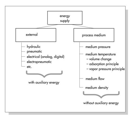
Fig. 3: Energy supply of control equipment
