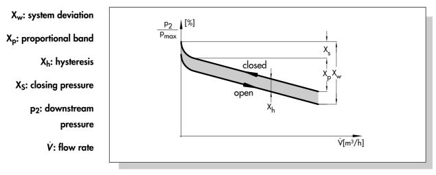
Fig. 9: Characteristic of a pressure reducing valve
