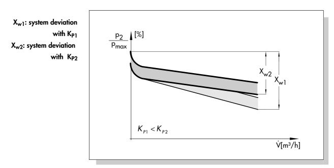
Fig. 10: System deviation with different proportional-action coefficients
