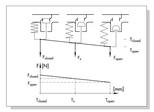
Fig. 6: Spring forces and characteristic
