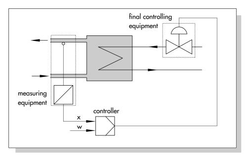
Fig. 1: Control loop with conventional instrumentation
