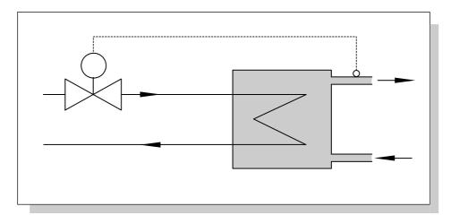
Fig. 2: Control loop with self-operated regulator
