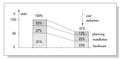
*Fig. 8: Cost reductions with fieldbus system* (*Dr. Rathje, Bayer AG: calculation example for PROFIBUS-PA*)
