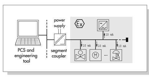
Fig. 4: Fieldbus system according to the FISCO model
