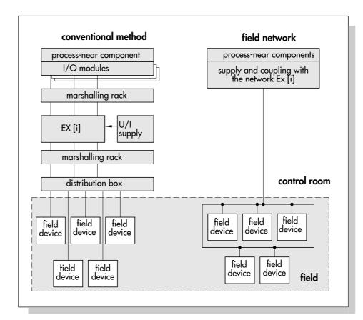
*Fig. 7: Comparison of conventional transmission method and field network wiring in hazardous areas*
