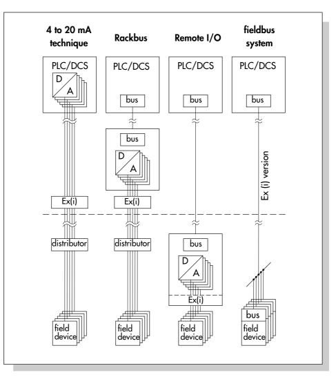
*Fig. 9: Rackbus and Remote I/O systems compared to conventional and fieldbus wiring*
