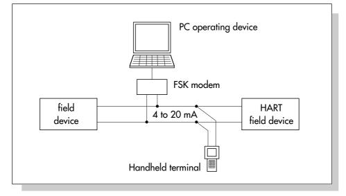
Fig. 6: Connection of HART field and operating devices
