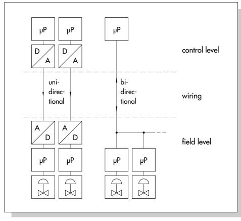
Fig. 1 Comparison of communication techniques: 4 to 20 mA technique vs. bus wiring with bidirectional communication
