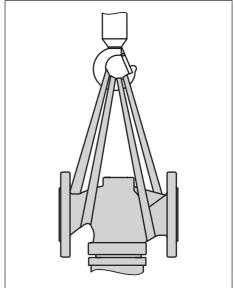
Fig. 4-1: Schematic drawing of lifting points on the regulator
