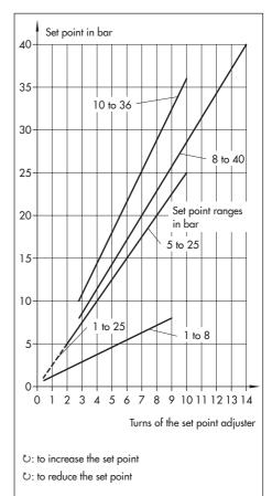
Fig. 2: Adjustment diagram
