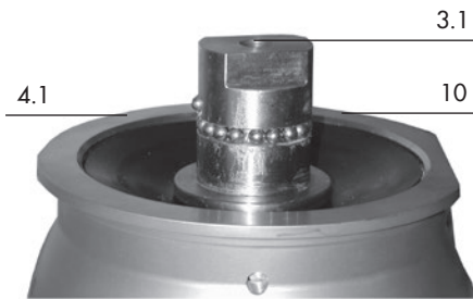
Actuator housing (10) with set point pressure port p_c and locking pin (16)
