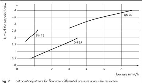
Fig. 9: Set point adjustment for flow rate: differential pressure across the restriction  $\Delta p_{restriction} = 0.2$  bar
