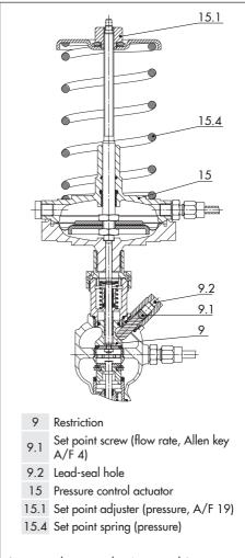
Fig. 7: Flow control · DN 15 and 25
