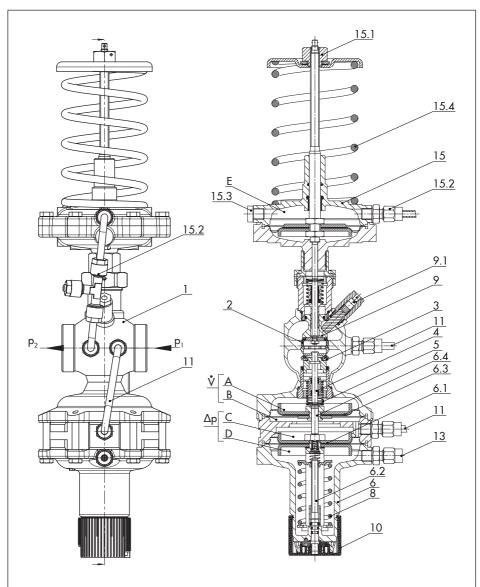
Fig. 2: Flow and differential pressure regulator with additional pressure control actuator · DN 15 and 25
