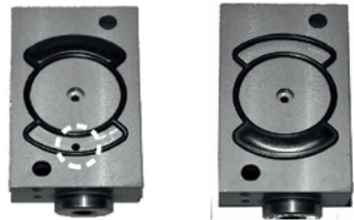
Fig. 8: CNOMO interface: location of the turnable gasket for internal air supply (left) and for external air supply (right)
