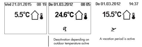
Fixed set point control · Current temperature = Flow temperature
