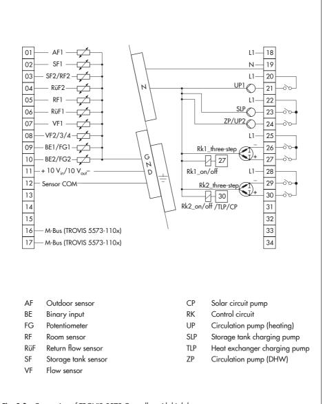
Fig. 5-3: Connection of TROVIS 5573 Controller with high base
