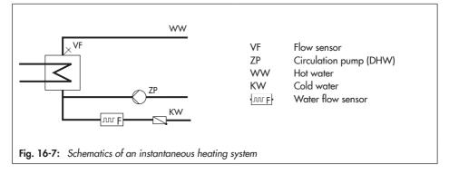
Without flow rate sensor or flow switch, the control of the required DHW temperature at the flow sensor VF is only active during times-of-use of the circulation pump ZP. The water flow sensor or flow switch allows the controller to recognize when DHW tapping starts and stops. Control of the required DHW temperature can made to be active only during DHW tapping by deleting all times-of-use of the circulation pump.
