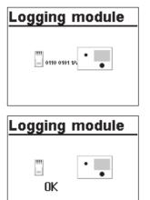
The data logging module is plugged into the RJ-45 connector socket located at the side of the controller. Once the module has been connected, 'Start data logging' and 'Copy logging data' appear on the controller display.
