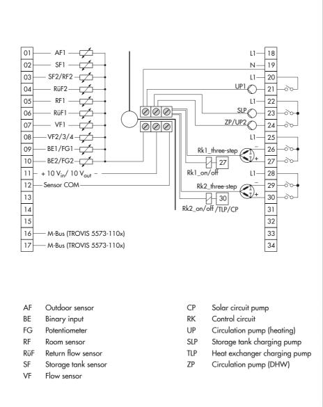
Fig. 5-2: Connection of TROVIS 5573 Controller with standard base
