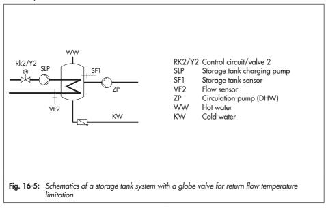
Globe valve and flow sensor VF2 are used exclusively for return flow temperature limitation in the schematics shown above. The pre-control circuit provides at least the same flow temperature as in the standard schematic version which is calculated from 'DHW temperature set point' + 'Charging temperature boost' + 'Boost set point (pre-control circuit)'.
