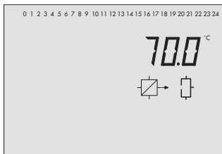
Flow sensor VF2, DHW circuit
