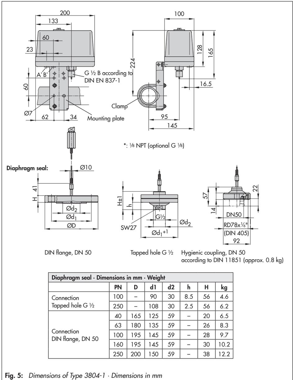
Fig. 5: Dimensions of Type 3804-1 · Dimensions in mm
