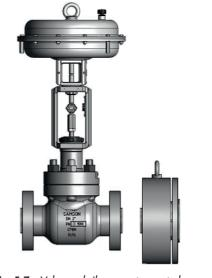
Fig. 5-7: Valve and silencer not mounted together, lifting eyelet on top
