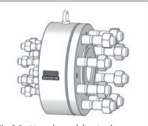
Fig. 2-3: Nameplate and directional arrow on the silencer
