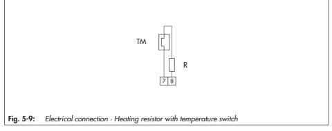
→ Connect the heating resistor R with temperature switch TW at terminals 7 and 8.
