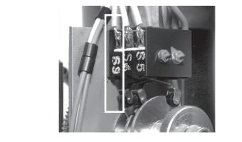
Fig. 7-8: Switch WE-S3 with associated cam disk
