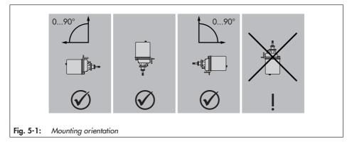
When the actuator is installed with the actuator stem in horizontal position, mount the yoke such that its two rods are positioned on top of each other in the vertical plane.
