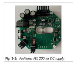
DIP switches and keys are used to select the required parameter settings.
