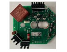
Fig. 3-4: Positioner PEL 200 for AC supply
