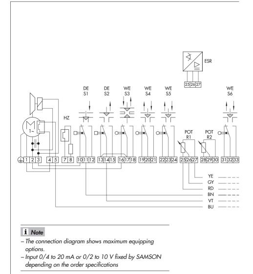
Fig. 5-13: Electrical connection · Version with positioner PEL 100 in single-phase operation
