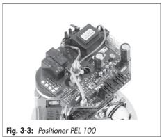
The travel calibration, split-range operation, reversed direction of action and dead band settings are changed using the potentiometers and switches (see Annex A).
