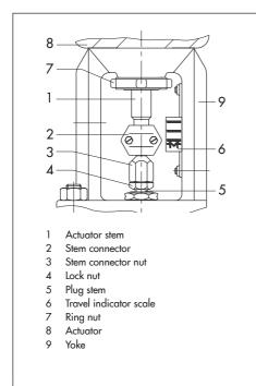
Fig. 5-3: Attachment to the valve
