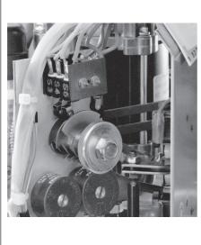
Fig. 3-6: Switches and resistance transmitters
