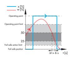
If the set point (---) is above 'Limit operating point' when the automatic mode starts, the valve (—) moves to the operating point. The valve moves back to the fail-safe position (0 % in the example) if the set point then falls below 'Limit fail-safe position'.
