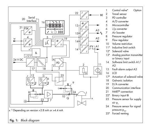
The positioner is fitted with three binary contacts as standard: A fault alarm output indicates a fault to the control room and two configurable software limit switches are used to indicate the end positions of the valve.
