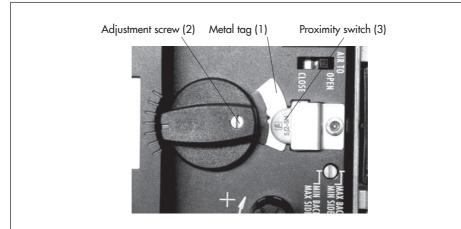
Fig. 38: Adjusting the limit switch
