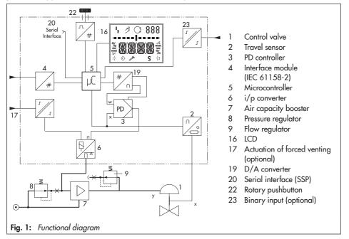
The fixed flow regulator (9) ensures a constant air flow to the atmosphere, which is used to flush the inside of the positioner housing and to optimize the air capacity booster (7). The i/p converter (6) is supplied with a constant upstream pressure by the pressure regulator (8) to compensate for any fluctuations in the supply pressure.
