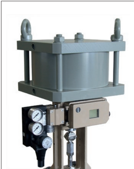
Fig. 7: Type 3710 Reversing Amplifier, Type 4708-54 Supply Pressure Regulator with Type 3730 Positioner mounted on Type 3275 Piston Actuator
