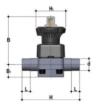
2-way diaphragm valve with stroke limiter and male ends for solvent respectively socket welding, metric series, code 39
