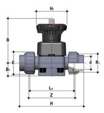
2-way diaphragm valve with **female union ends** for solvent welding, **BS series**, code 31
