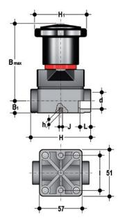
Compact diaphragm valve with **female ends** for solvent respectively socket welding, **metric series**, code 2
