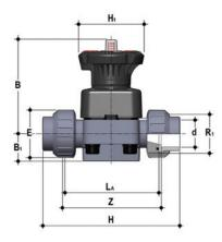
2-way diaphragm valve with **female union ends** for solvent respectively socket welding, **metric series**, code 30
