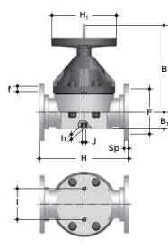
2-way diaphragm valve with fixed flanges, drilled PN10/16. Face to face according to EN 558-1, code 81
