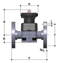
2-way diaphragm valve with fixed flanges, drilled PN10/16. Face to face according to EN 558-1, code 81
