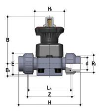
2-way diaphragm valve with stroke limiter and female union ends for solvent respectively socket welding, metric series, code 30
