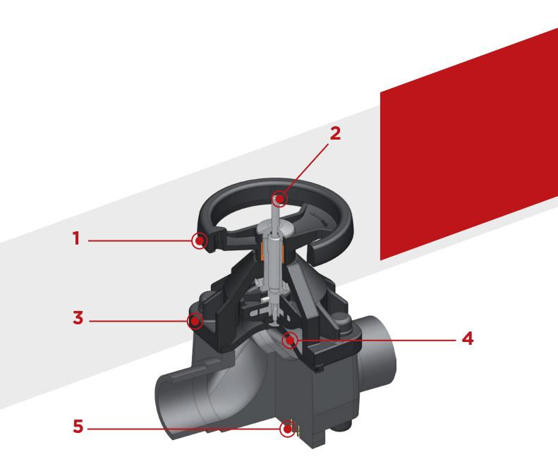
Handwheel in (PP-GR) with high mechanical strength and ergonomic grip for optimum manageability
