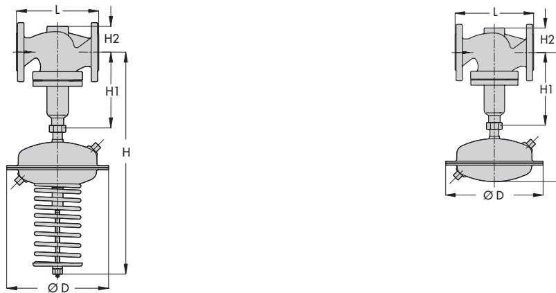
Type 42-24 · Type 2422 Valve balanced by a bellows with Type 2424 Actuator Type 42-28 · Type 2422 Valve balanced by a bellows with Type 2428 Actuator
