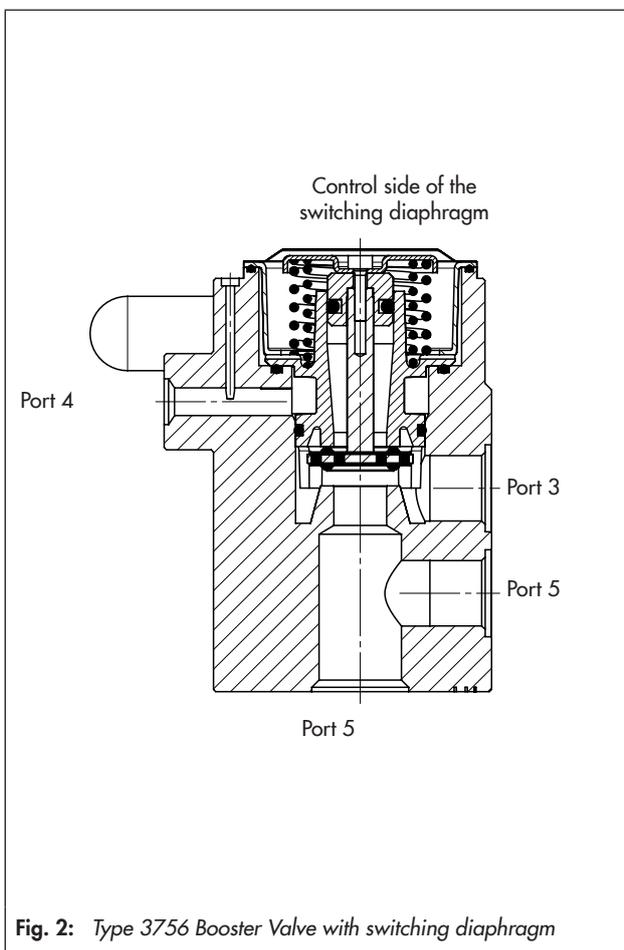
Fig. 2: Type 3756 Booster Valve with switching diaphragm
