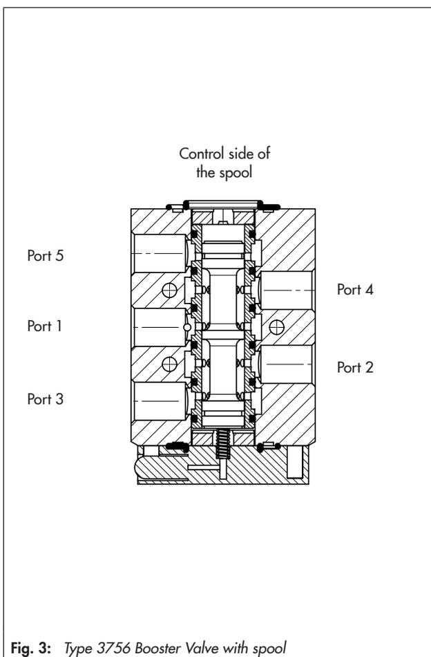
Fig. 3: Type 3756 Booster Valve with spool
