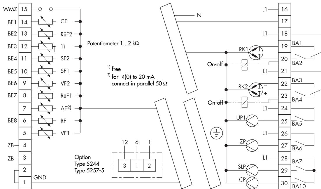
Fig. 9 · Terminal assignment for system code no. 5
