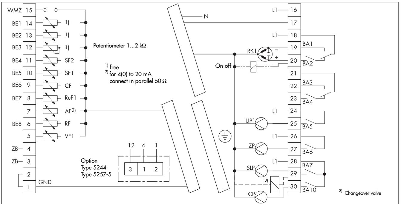
Fig. 8 · Terminal assignment for system code no. 2
