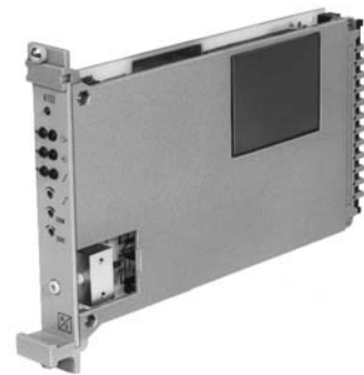
Fig. 1 · Type 6132-01 p/i converter, rack-mounting unit
