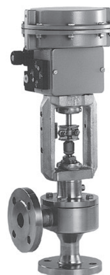
Fig. 2: Type 3249-7 Control Valve in special version with backup packing, bar stock body with flanges, Type 3277-5 Pneumatic Actuator and integrated Type 3767 Electropneumatic Positioner
