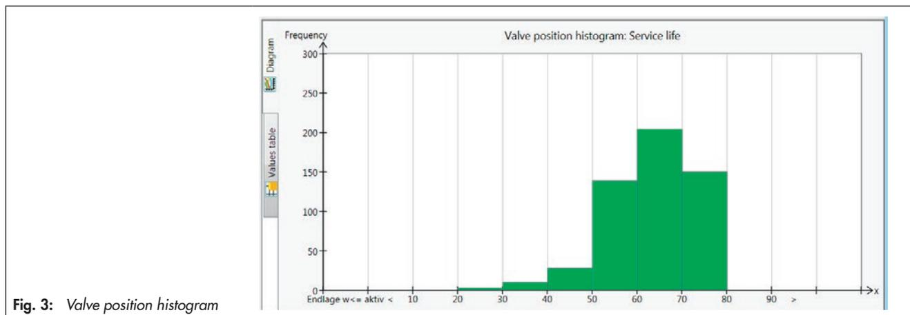
Fig. 3: Valve position histogram
