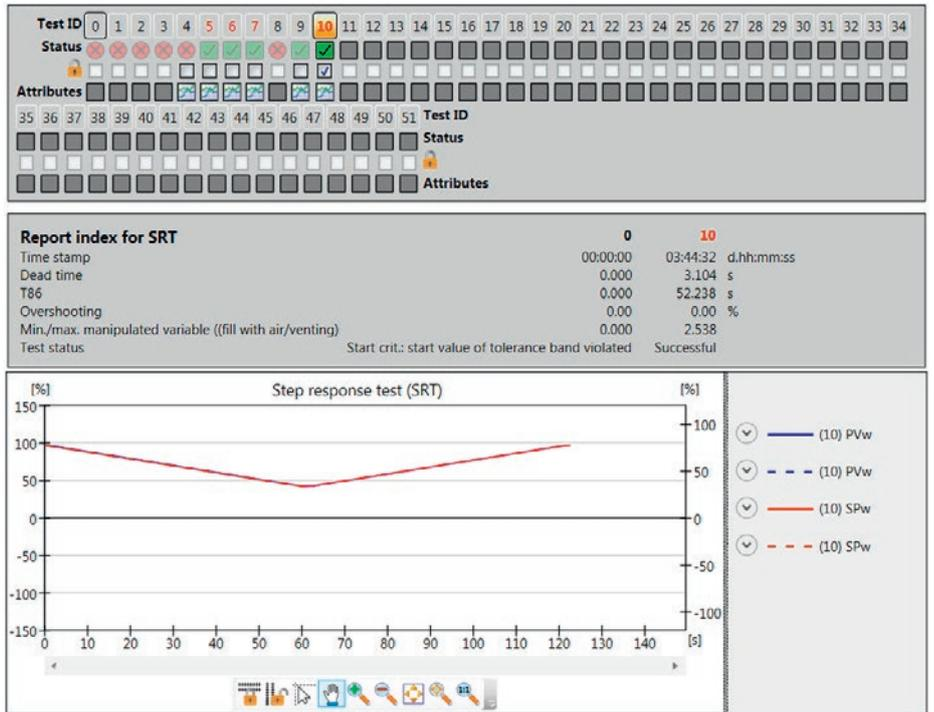
Fig. 8: Step response test (SRT)
