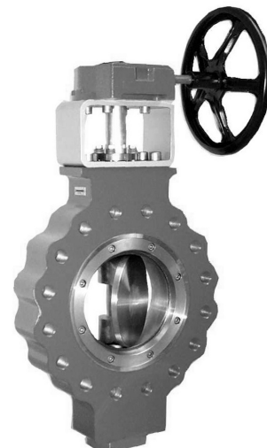
Fig. 2 · Tight-closing Type LTR 43 Butterfly Valve, lug-type, metal sealing with manual gear
