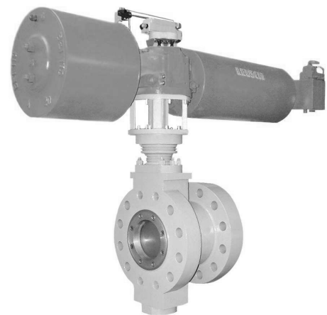
Fig. 1 · Type LTR 43 High-pressure Butterfly Valve in double-flanged version, NPS 10, Class 1500 with pneumatic actuator and positioner
