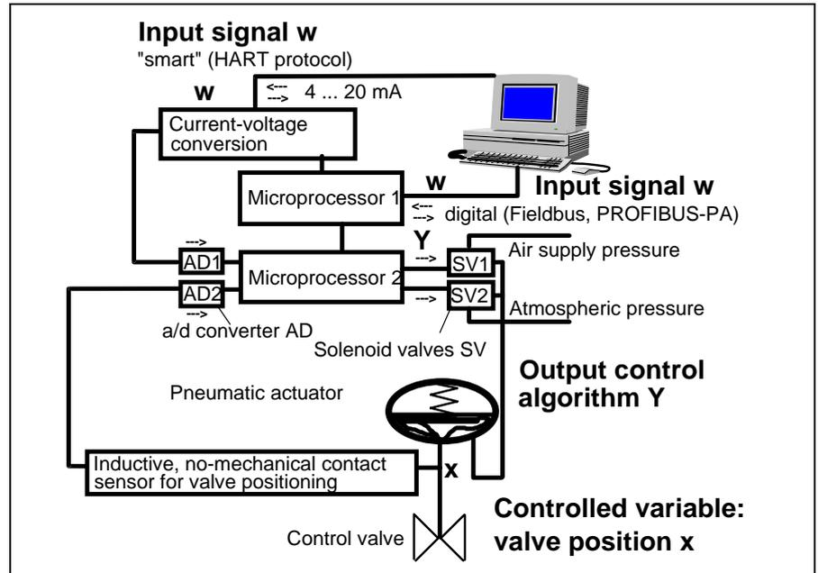
Fig. 3: Digital positioner design (SAMSON Types 3780/3781/3785)
