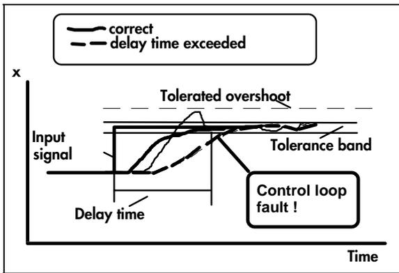
Fig. 6: Supervising the control loop of digital positioners
