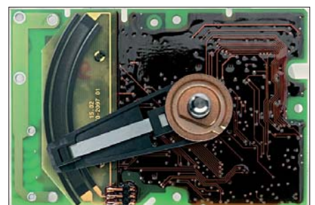
Fig. 4: Potentiometer as position sensor
