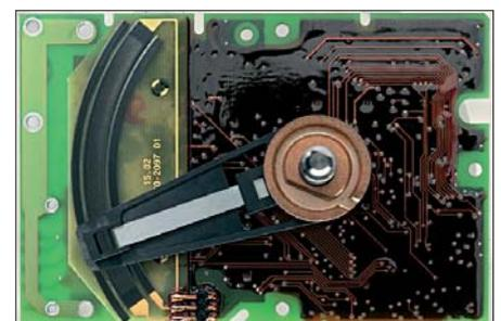
Fig. 4: Potentiometer as position sensor
