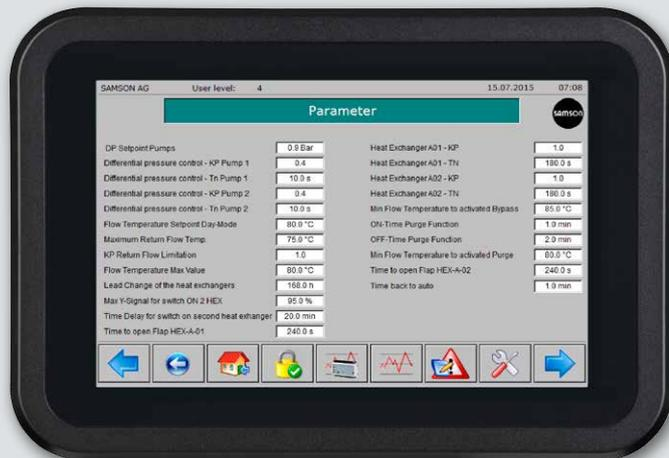
Fig. 4: Overview of parameters on the TROVIS 6616 Web Terminal
