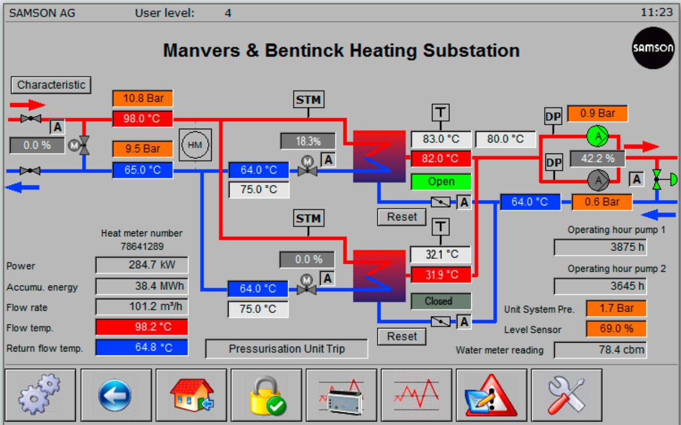
Fig. 1: Hydraulic scheme of the plant
