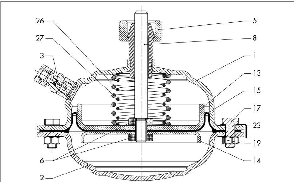
Fig. 15-5: Type 2426 Diaphragm Actuator, DN 15 to 250
