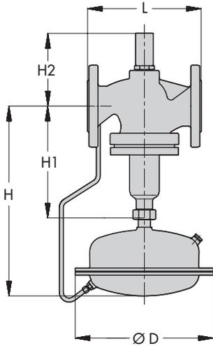
Type 2423 Valve, balanced by a diaphragm
