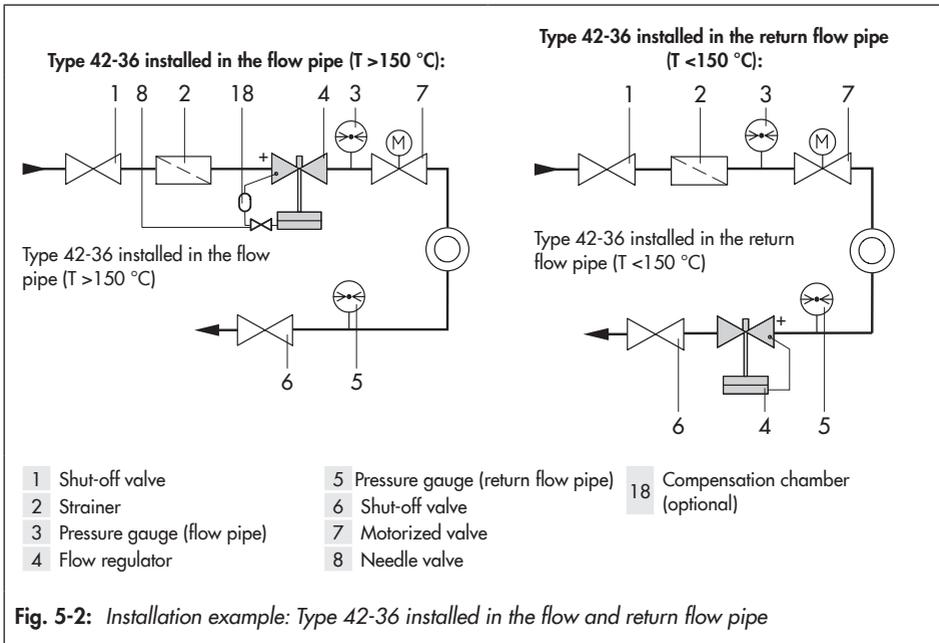
Fig. 5-2: Installation example: Type 42-36 installed in the flow and return flow pipe
