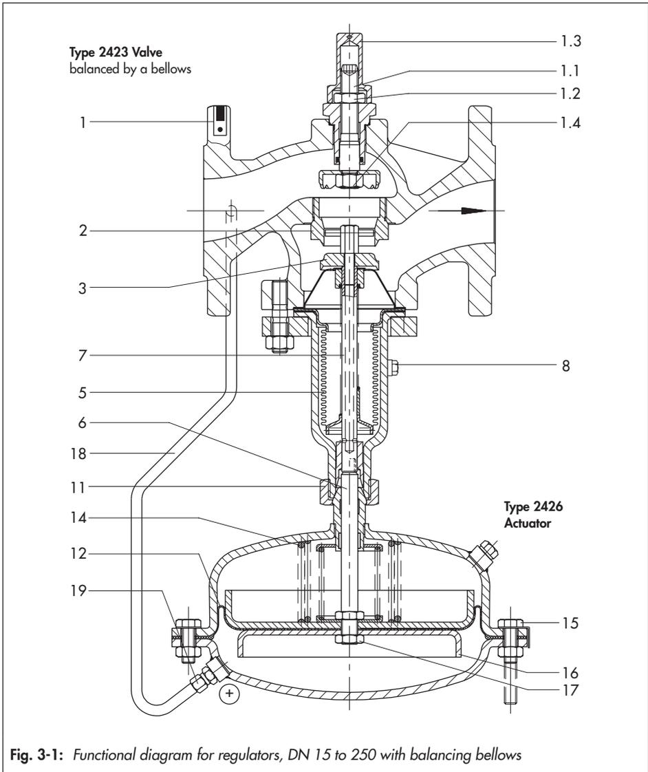
Fig. 3-1: Functional diagram for regulators, DN 15 to 250 with balancing bellows
