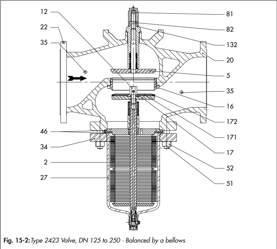
Fig. 15-2: Type 2423 Valve, DN 125 to 250 · Balanced by a bellows
