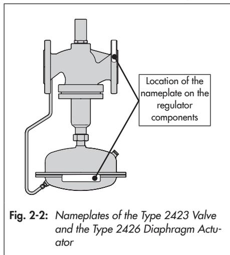
**Fig. 2-2:** Nameplates of the Type 2423 Valve and the Type 2426 Diaphragm Actuator
