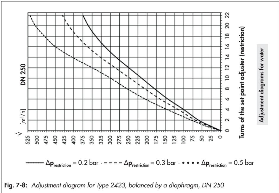
Fig. 7-8: Adjustment diagram for Type 2423, balanced by a diaphragm, DN 250
