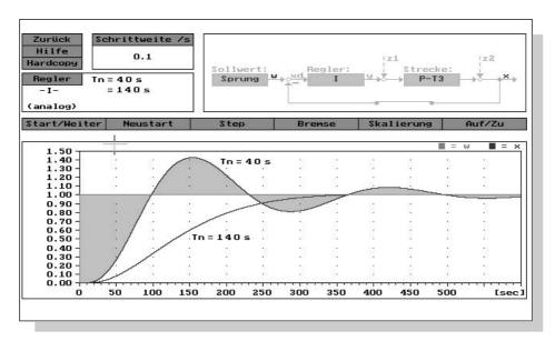
Fig. 31: Control response of the I controller with PT<sub>3</sub> system (double time scale)
