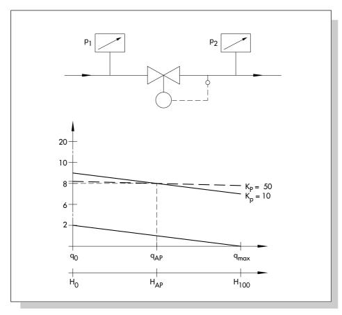
Fig. 26: Functional principle and characteristics of a pressure reducing valve
