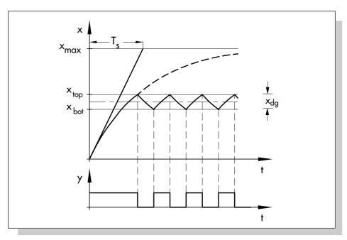
Fig. 42: Control cycle of a two-position controller with differential gap and first-order controlled system
