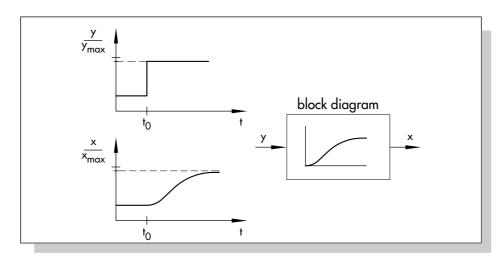
Fig. 11: Dynamic behavior of second- or higher-order controlled systems (y: valve position; x: medium temperature in the second tank)
