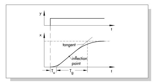
Fig. 12: Step response of a higher-order controlled system with the characteristic values  $T_u$  and  $T_g$
