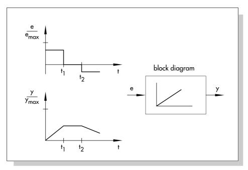
Fig. 30: Dynamic behavior of an I controller (e: system deviation; y: manipulated variable)
