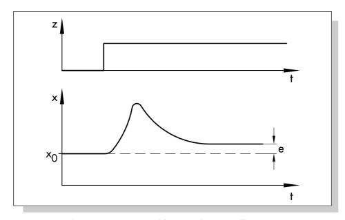
Fig. 25: Steady-state error in control loops with P controllers  $x_0$ : adjusted operating point of the controller
