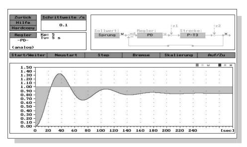
Fig. 34: Control response of the PD controller with PT<sub>3</sub> system
