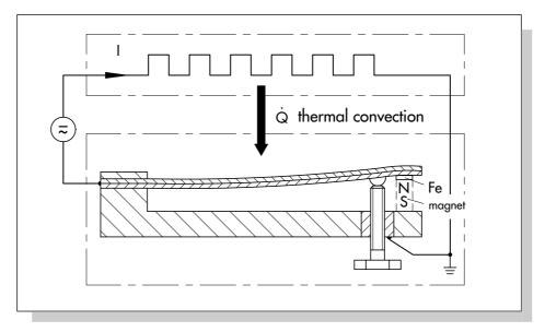
Fig. 43: Temperature control via bimetallic switch
