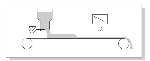
Fig. 5: Controlled system with dead time
