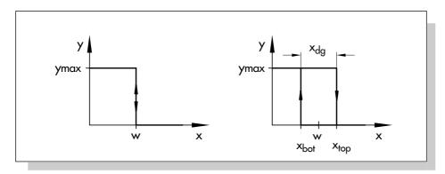
Fig. 41: Switching charakteristic of the two-position controller (without and with differential gap  $x_{dg}$ )
