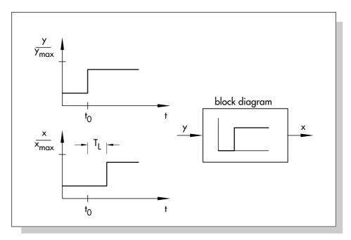
Fig. 6: Dynamic behavior of a controlled system with dead time (y: slide gate position; x: conveying quantity)
