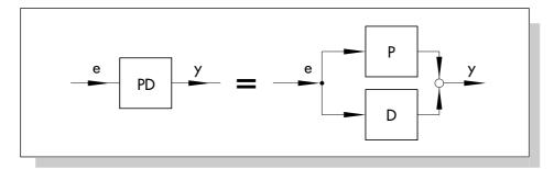
Fig. 32: Elements of a PD controller
