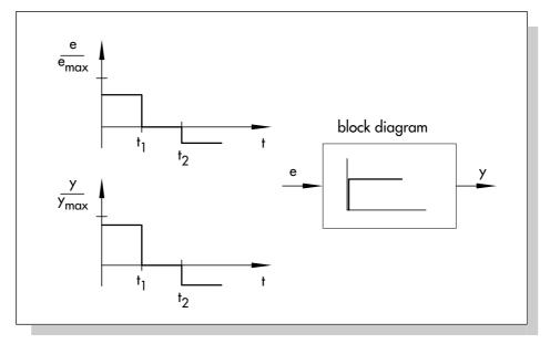
Fig. 23: Dynamic behavior of a P controller (e: system devitation; y: manipulated variable)
