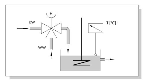
Fig. 8: First-order controlled system; controlled variable: temperature
