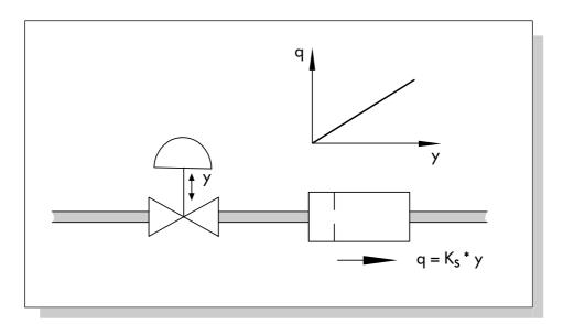
Fig. 1: Proportional controlled system; reference variable: flow rate
