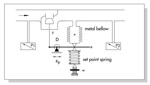
Fig. 22: Design of a P controller (self-operated regulator)
