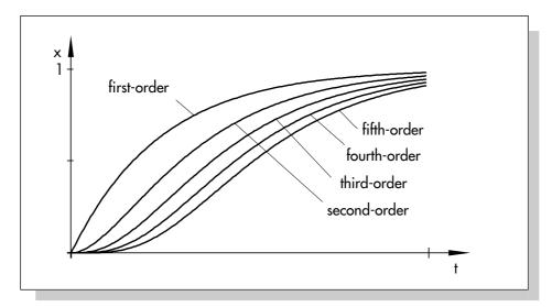
Fig. 13: Dynamic behavior of higher-order controlled systems
