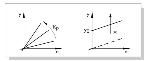
Fig. 24: Effect of K<sub>P</sub> and operating point adjustment
