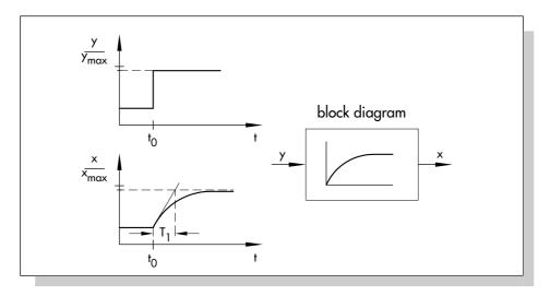
Fig. 9: Dynamic behavior of a first-order controlled system –  $PT_1$  element (y: valve position; x: temperature of liquid in tank)
