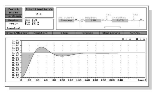
Fig. 40: Control response of the PID controller with PT<sub>3</sub> system
