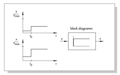
Fig. 2: Dynamic behavior of a P controlled system (y: control valve travel; x: flow rate in a pipeline)
