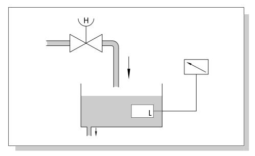
Fig. 3: Integral controlled system; controlled variable: liquid level in a tank
