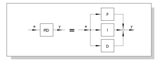
Fig. 38: Elements of a PID controller
