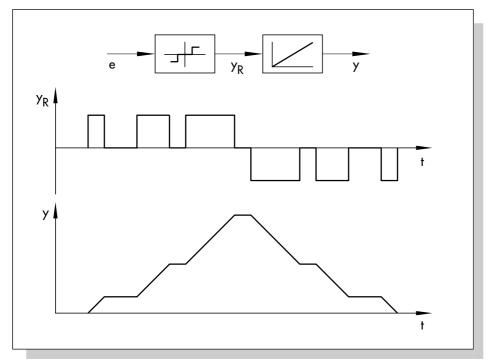
Fig. 46: Control signal of a quasi-continuous controller (three-position controller with actuator motor)
