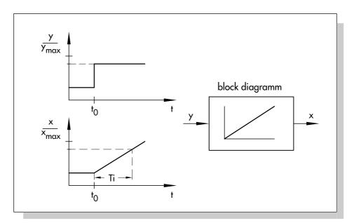
Fig. 4: Dynamic behavior of an I controlled system (y: valve travel; x: liquid level in a tank)
