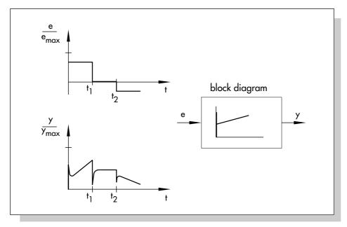
Fig. 39: Dynamic behavior of a PID controller (e: system deviation; y: manipulated variable)
