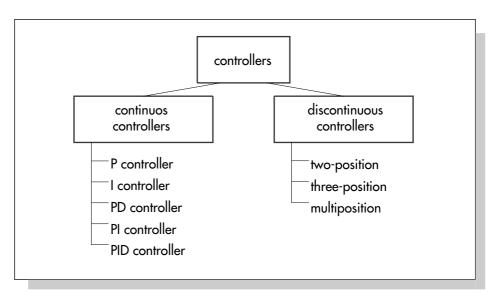
Fig. 18: Classification of controllers
