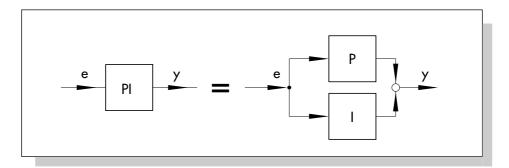
Fig. 35: Elements of a PI controller
