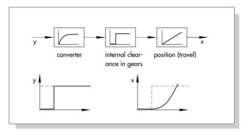
Fig. 14: Dynamic behavior of an actuator with internal clearance in its gears (lagging integral response with dead time)
