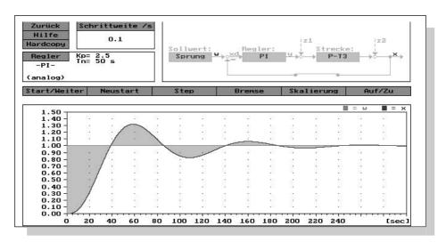
Fig. 37: Control response of the PI controller with PT<sub>3</sub> system
