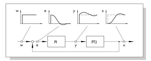
Fig. 20: Signal responses in a closed control loop
