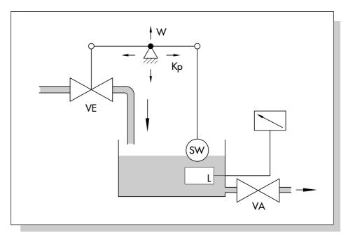
Fig. 27: Level control with a P controller (self-operated regulator)
