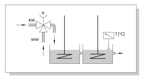
Fig. 10: Second-order controlled system; controlled variable: temperature
