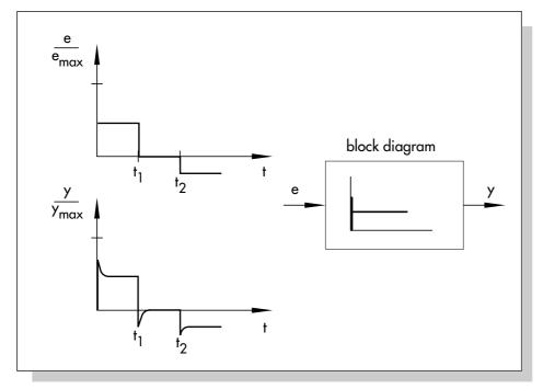
Fig. 33: Dynamic behavior of a PD controller (e: system deviation; y: manipulated variable)
