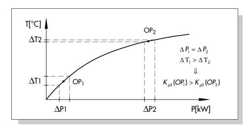
Fig. 16: Operating point-dependent behavior of the steam-heated tank
