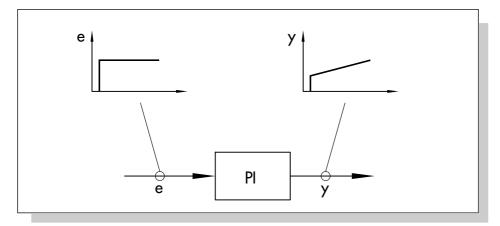
Fig. 19: Step response of a controller
