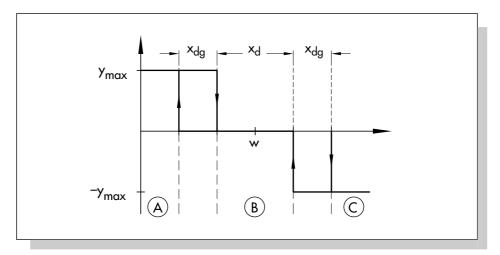
Fig. 45: Characteristic of a three-position controller with differential gap  $x_{dg}$  and dead band  $x_d$
