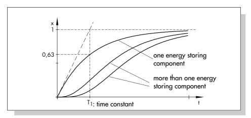
Fig. 7: Exponential curves describe controlled systems with energy storing components
