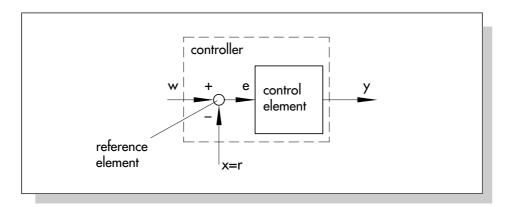
Fig. 17: Controller components
