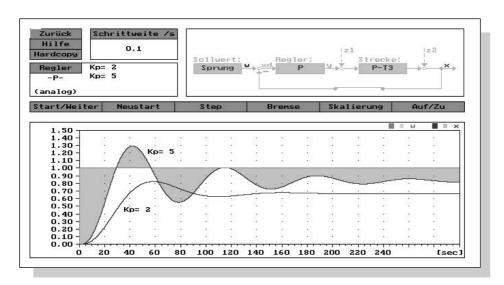
Fig. 28: Control response of the P controller based on a PT<sub>3</sub> system
