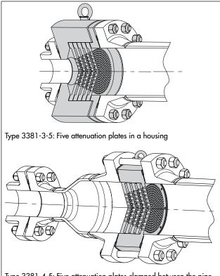
Type 3381-4-5: Five attenuation plates clamped between the pipe expander and pipeline (wafer-type version)
