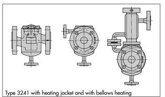
A heat transfer medium flowing between valve body and heating jacket ensures that the process medium is kept at a certain temperature. If steam is used as heating transfer medium, proper condensate discharge must be ensured.
