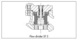
The valve-specific correction values for gases and vapors are required for noise calculation according to VDMA 24422, Edition 1989 and IEC 60534 when flow dividers are used. Refer to the diagrams in section 'Calculation of noise emission' for details.
