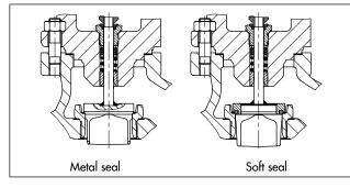
The seat, plug and plug stem are made of stainless steel. In some cases, the trims are subject to high stress due to high differential pressures, cavitation, flashing or in cases where the process media contains solids. In order to increase the service life, seats and metal-seated plugs can have a Stellite<sup>®</sup> facing and plugs up to DN 100 can be made of solid Stellite<sup>®</sup>.
